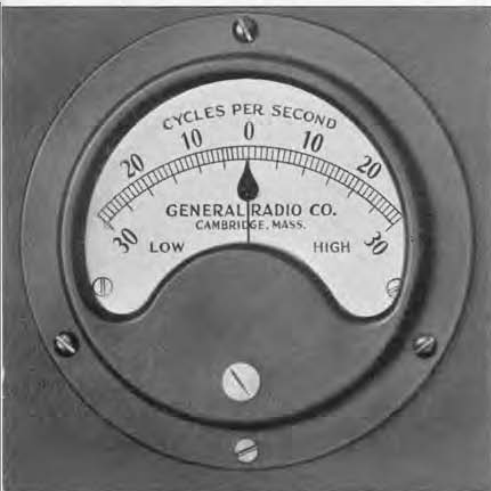
FIGURE 6. Frequency deviations are indicated on this meter, which can be read to better than one-half cycle.
