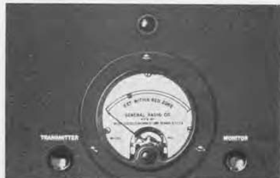
FIGURE 4. The signal-level indicator on the frequency monitor unit. When the input level is correct, the meter reading is within the red (shown black in the photograph) range on the scale.
